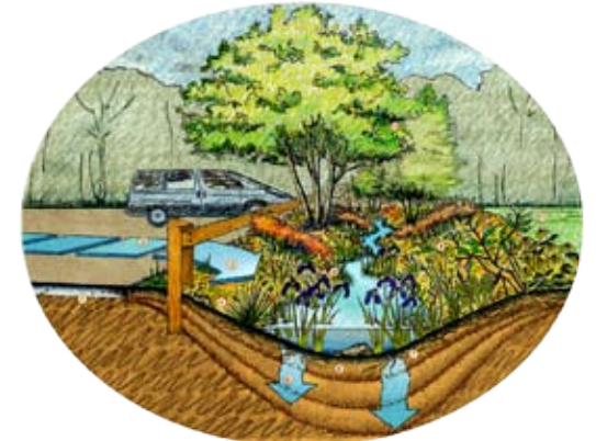
Parking drainage swale - The parking areas for the Montgomery Street area should incorporate landscaping combined with runoff management designs that naturally filter the storm waters. It is important for the Botanic Garden to set the example for sustainable landscapes.
